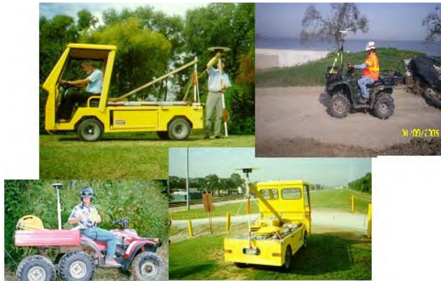
Figure 6-5. New Orleans District levee profiling using real-time kinematic GPS methods (New Orleans District and 3001, Inc.)
