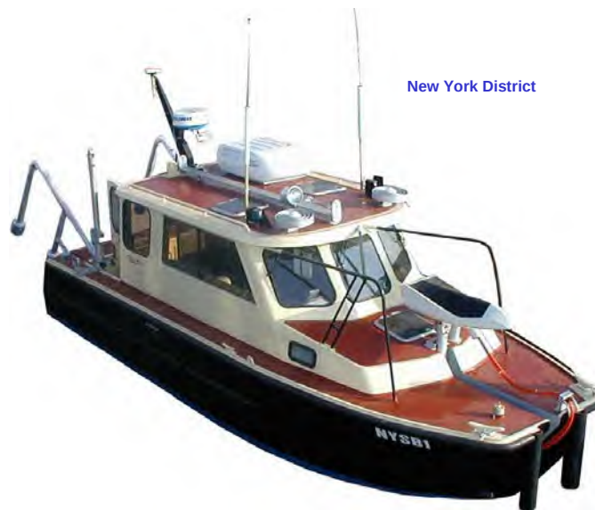
Figure 6-7. Typical Corps hydrographic survey vessel equipped with carrier phase DGPS and IMU for measuring vessel position, roll, pitch, and heave parameters during real-time surveys (New York District)
